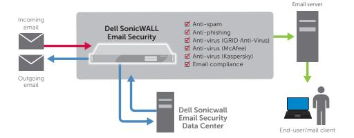
High availability deployment (Figure 2) For load balancing and redundancy, split mode enables organizations to filter at the network perimeter while providing centralized control. Administrators can easily synchronize Dell SonicWALL Email Security across multiple LDAP servers in distributed and hosted environments, for scalable deployment and flexible Try and Buy implementations.
