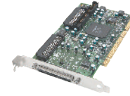
Adaptec SCSI Card 29320A-R 1-channel, 64/133 MHz, full-height, half-length card with HostRAID™ RAID 0, 1, and 10
