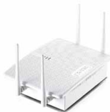
NWA5560-N 802.11 a/b/g/n Dual-Radio Managed Access Point
