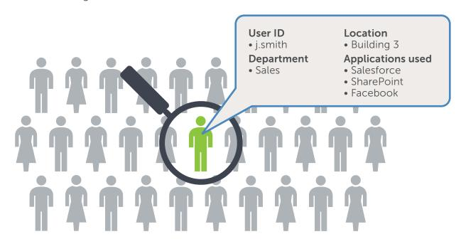
Active directory can be integrated into the IPS to tie applications used on the network to specific user credentials.
